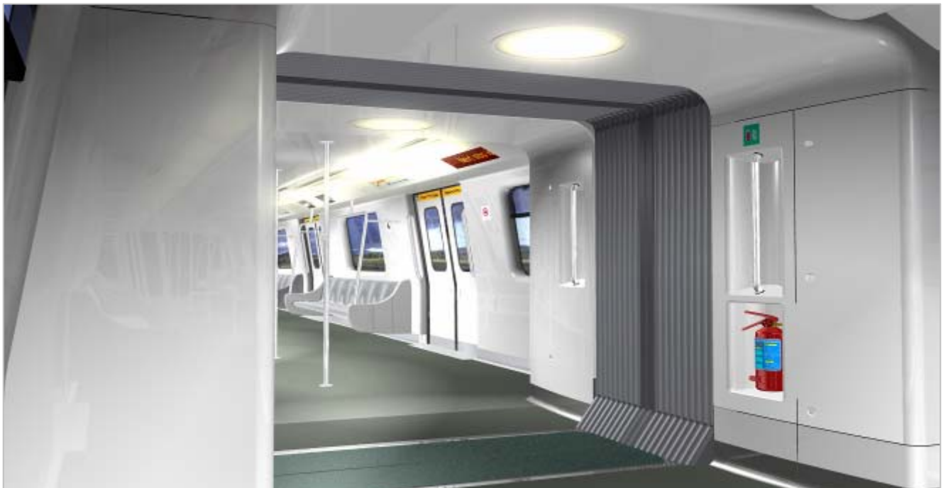
Figure 3.8: Gangways in Metro Rail
