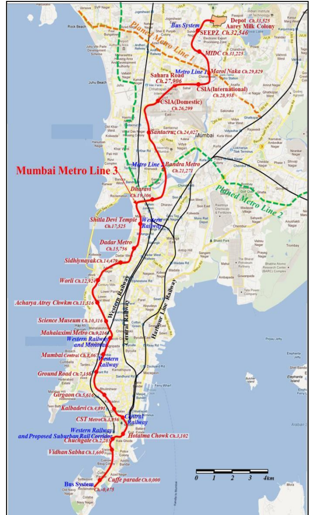
Figure 1: Alignment of Mumbai Metro Rail Line 3
