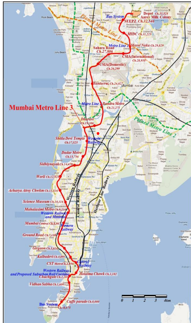
Figure 1: Alignment of Mumbai Metro Rail Line 3
