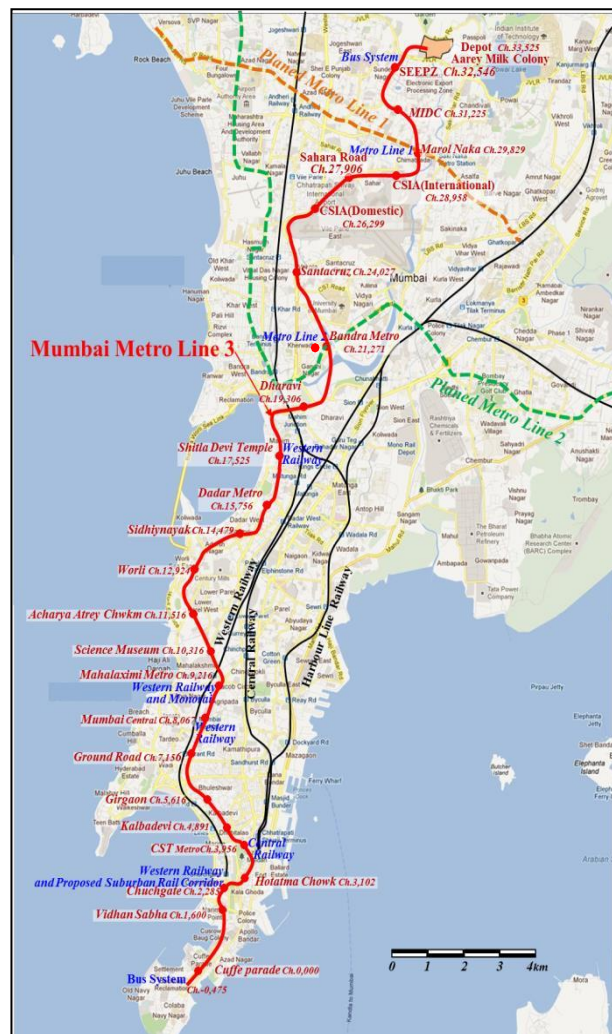
Figure 1: Alignment of Mumbai Metro Rail Line 3
