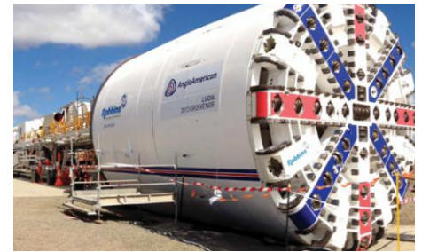
Package 3 TBM - Slurry
