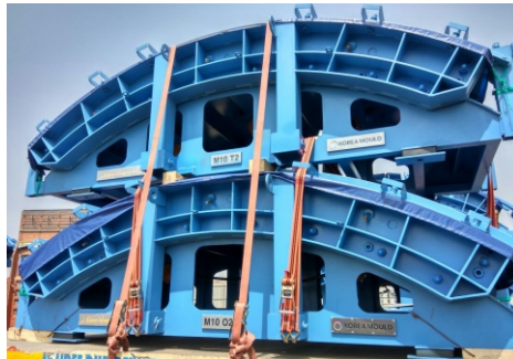
Imported segment ring casting mould from Korea
