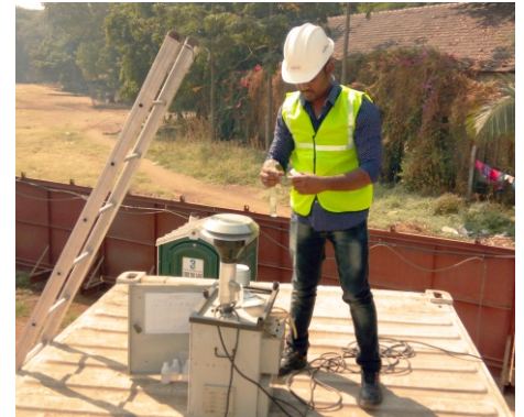
Ambient Air Quality test using respirable dust sampler Azad Maidan
