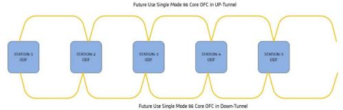
b. The 96-core single mode Future use cable of FOTS-FO system is laid and terminated in all stations as shown in above figure. This cable is laid in both Up-Tunnel & Down tunnel and all the 96 cores will be terminated in TER FDMS.
