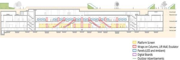
Note: Mumbai Metro Line 3, being a fully underground line, will have external facade limited to the extent of the entry / exits to the stations.
