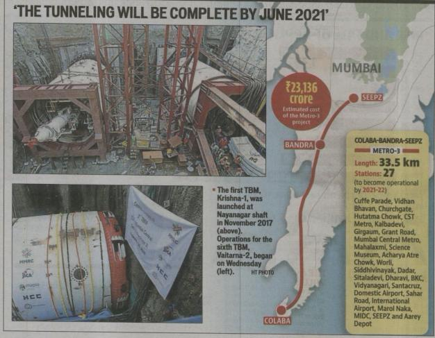
"When we lower the machine inparts, we start the initial drive. Once it is lowered completely, it is called the main drive," Bhide explained.
