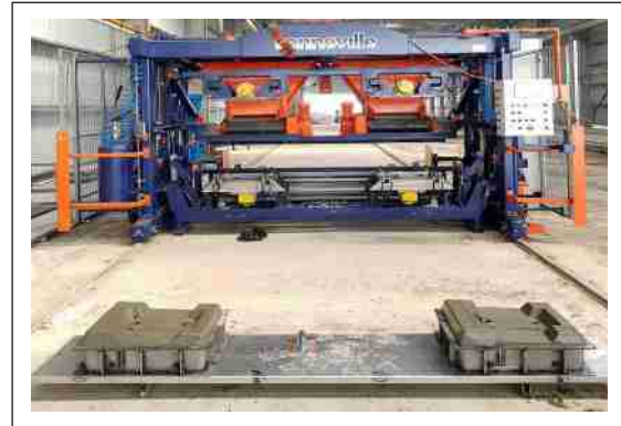
Sleeper Block Machine being used to cast blocks at Wadala Cating Yard for Line 3 11.11.2020
